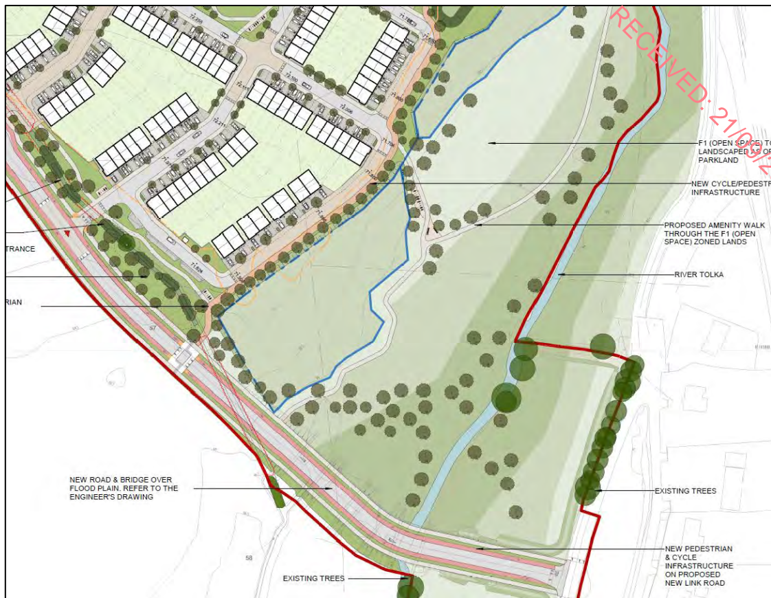
Figure 13.29. Image extracted from the Landscape Design Context Plan (irla Drwg: 1000) showing the proposed new network of hedgerow/tree planting linking the south of the Site with the Tolka riparian corridor.
