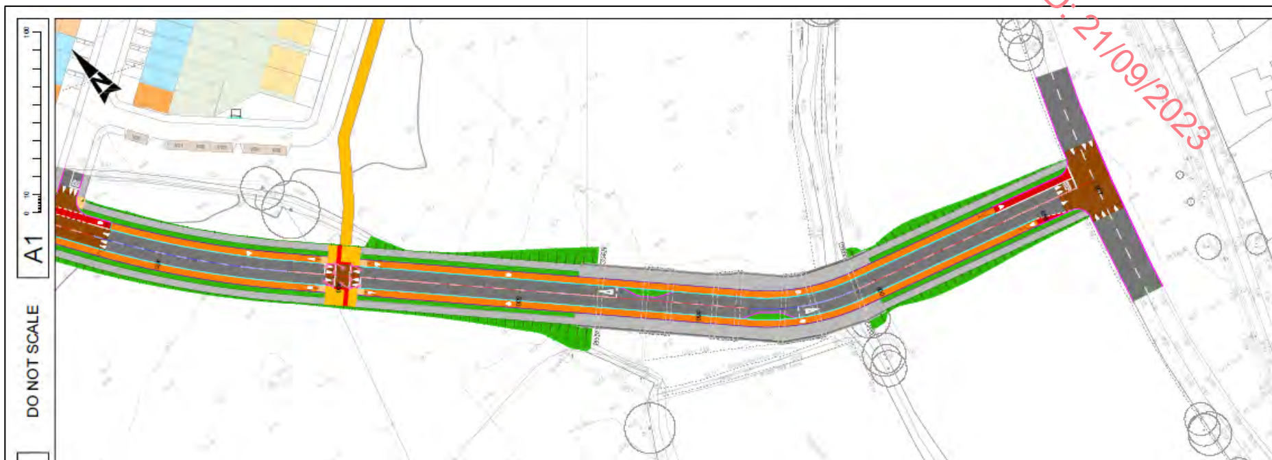
Figure 13.7. Image extracted from Atkins Drwg no: 5205505-ATK-ZZ-ZZ-SK-CE-000025, showing the southern Link-road as it crosses the Tolka and flood plain.
